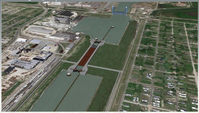
New 900 feet long by 110 feet wide IHNC Lock, with a sill elevation of -22.0 feet NAVD88.
