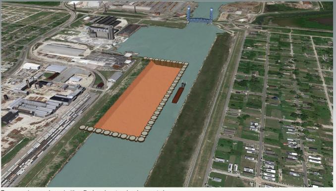
Temporary bypass channel with cofferdam dewatered and excavated.
