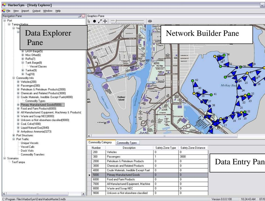
HarborSym has additional windows into its functionality to increase user confidence and understanding. A within simulation animation provides detailed information on how the model is applying rules. This visualization is provided as the model computes vessel locations and interactions, and the user can pause the simulation to retrieve additional data on elements within the system.
