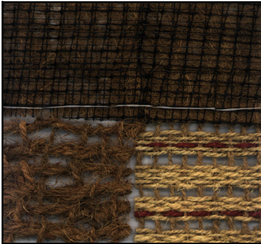
Erosion Control Blankets
