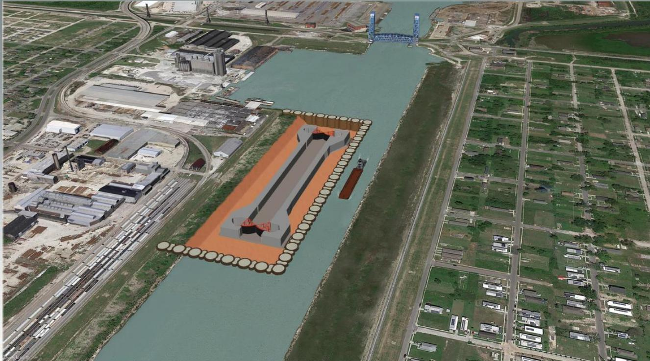
Cofferdam with sector gate and lock constructed.
