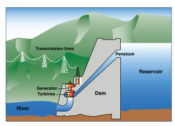
Just having water in the river isn't enough. A good hydropower site must have enough streamflow as well as enough head. For example, the Mississippi River has tremendous streamflow, but only a few of its dams are high enough to provide the head needed for efficient hydropower development. Dams in the arid West may have plenty of head, but not enough streamflow. Where the right combination of streamflow and head exists, the Corps has included powerplants at its dam.
