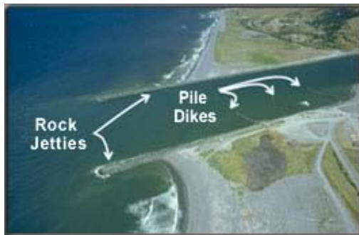
Figure A-5: Jetties and Pile Dikes
