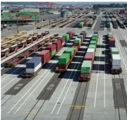
Figure 8. Double stacking containers on railroad cars is one of numerous tactics used to reduce rail transport costs and decrease atmospheric emissions per ton transported.
