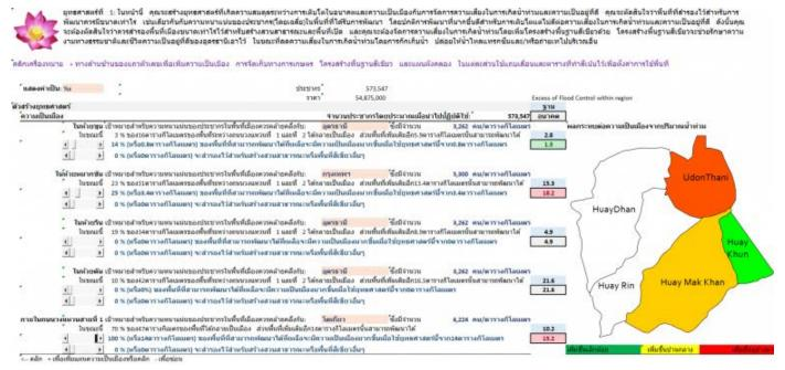
This graphic shows one of the shared vision planning model interfaces which allows negotiations between the various interests in locating and sizing green infrastructure to regulate, store, or route flood waters.
