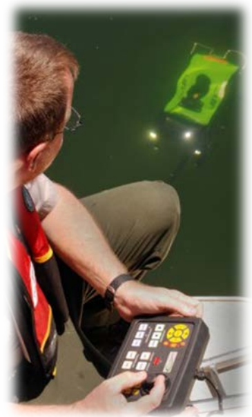
"Flying" the underwater robotic vehicle to surface near the work boat, Ranger John Chapman, U.S. Army Corps of Engineers Sacramento District (Photo: Robert Kidd)
