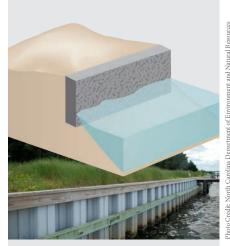
Parallel to the shoreline, vertical retaining wall. Intended to hold soil in place and allow for a stable shoreline.
