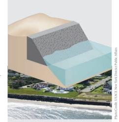
Parallel to shoreline, vertical or sloped wall. Soil on one side of wall is the same elevation as water on the other. Absorbs and limits impacts of large waves and directs flow away from land.
