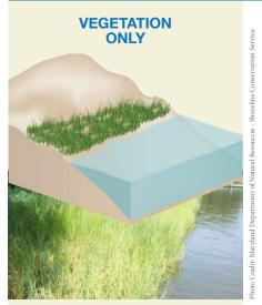
Roots hold soil in place to reduce erosion. Provides a buffer to upland areas and breaks small waves.
