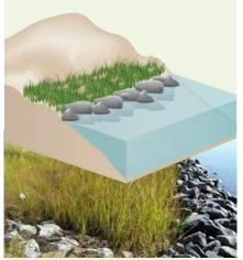
Parallel to existing or vegetated shoreline, reduces wave energy and prevents erosion. A gapped approach would allow habitat connectivity, greater tidal exchange, and better waterfront access.
