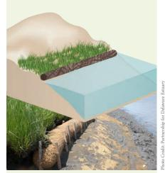
Structure to hold the toe of existing or vegetated slope in place. Protects against shoreline erosion.
